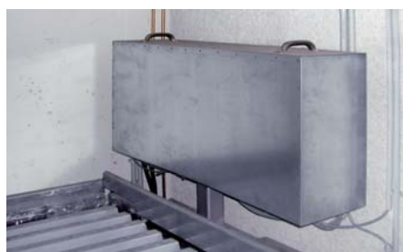
Sound insulation hood for the power unit
